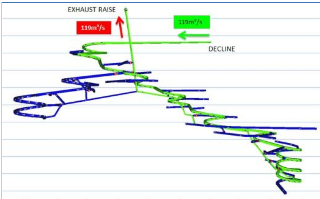
Figure 18.9: Ventilation Circuit in Phase 2 of Production
