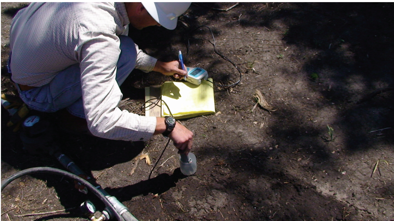
Photo 1 - UEC personnel taking water samples and measuring flow rates from one of its monitor wells at Goliad.
